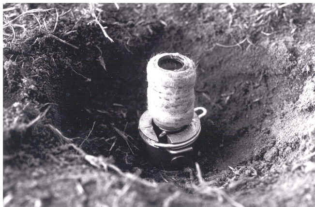
Figure 1. A set M-44 ready for baiting. The top (capsule holder) is wrapped or covered with an absorbent material, such as cheesecloth as shown here, to which an attractant lure or scent will be applied.
