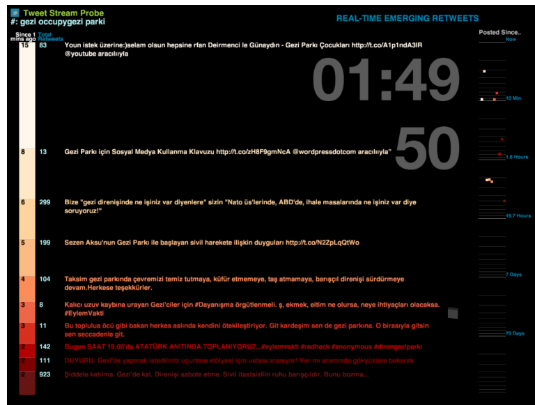
Figure 6.8: A screen shot of the real-time emerging retweet visualization. The animation on the left represents the number of new updates for each message since the application(TweetProbe) launched. Each segment and its corresponding message is color-coded with the square marker on the timeline graph, which is on the right side of the screen. The timer in the upper-right region of the screen shows the time elapsed since the program has been launched and the number below ('50') is the total number of new retweets since the launch of application.)
