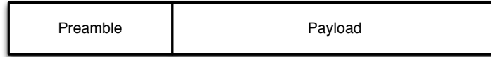
Figure 1.1: Packet format: The preamble is used for performing the synchronization operations such as code acquisition, carrier recovery and frame synchronization. The payload contains the useful data for communication.
