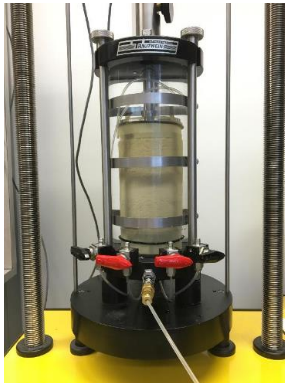
Figure 6.7 Consolidated drained triaxial compression test setup.
