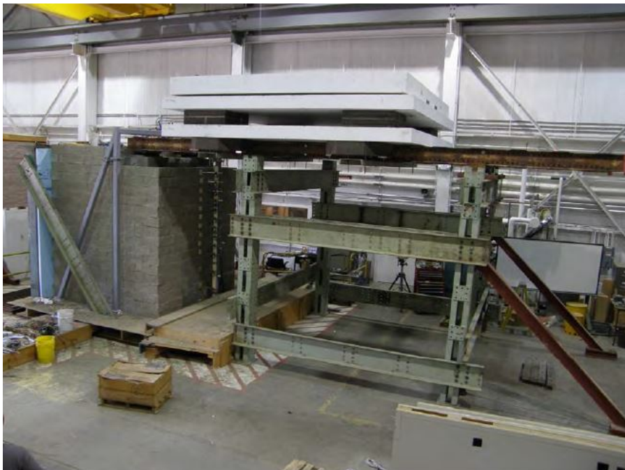
Figure 2.8 Shaking table test setup for GRS bridge abutment (from Helwany et al. 2012).
