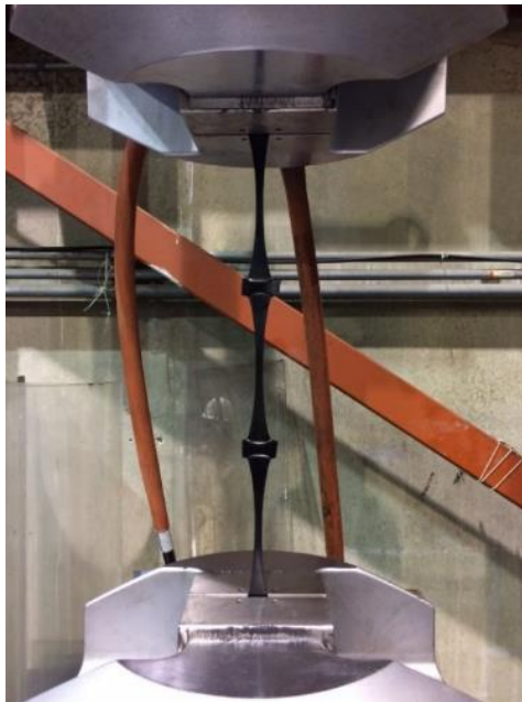
Figure 6.11 Single rib tensile test setup.
