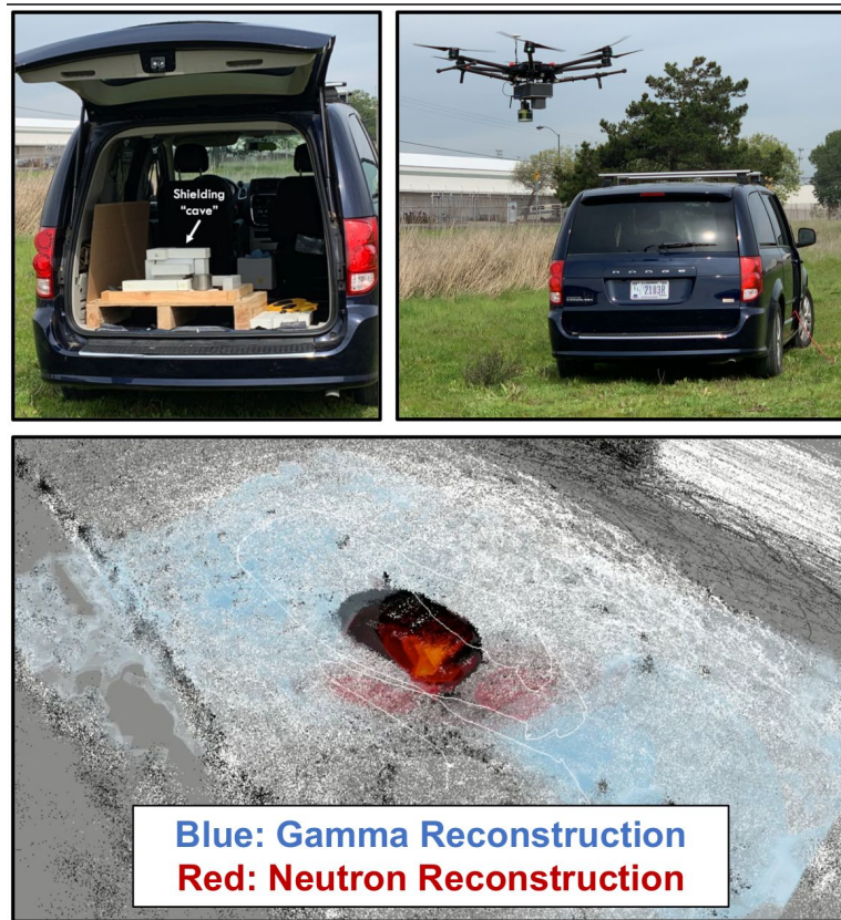
Figure 6: NG-LAMP reconstruction of simultaneous 3D real-time mapping of a shielded neutron source in the back of a vehicle. There are approximately 14 cm of lead and tungsten for shielding of a 1 SQ Pu surrogate source, which reduces the dose rate from gamma-ray emission, measured at the bumper, to about 10 \mu\text{R/hr} . Thus the source emission is considered to be purely neutrons. The reconstruction is consistent with the uniform background gamma-ray distribution, shown in blue, and the neutron distribution shown in red.
