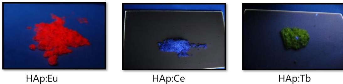
Figure 11. Emission of the HAp:RE powder under UV light.
