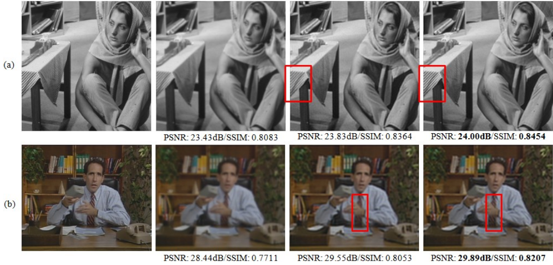
Figure 6.5: Conventional vs. cascade regularization on real-world images. (First column) Original. (Second column) Blurred. (Third column) Conventional. (Fourth column) Cascade. (a) Barbara. (b) Salesman.
