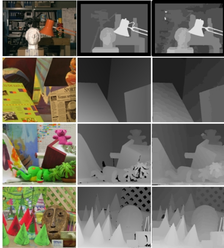
Figure 3.12: Disparity maps for “Tsukuba”, “Venus”, “Teddy” and “Cones”. Centered column shows ground-truth disparity map and right-most column shows the disparity map from the proposed algorithm.
