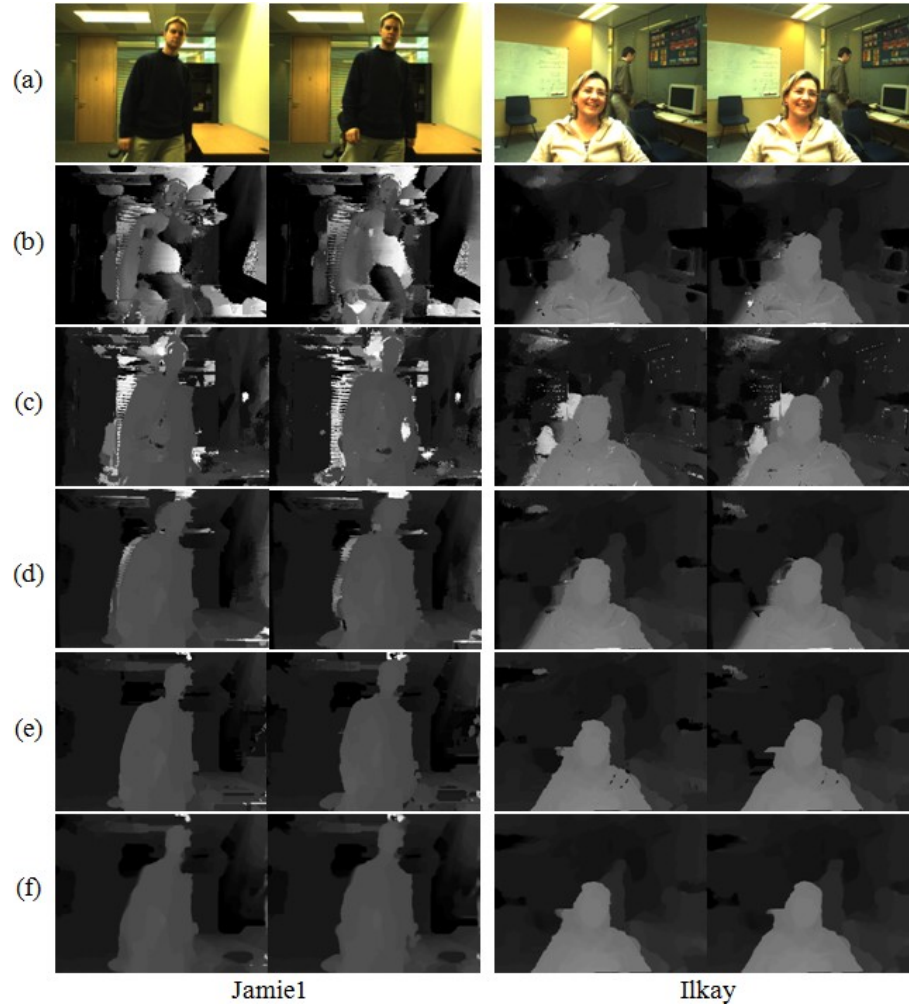
Figure 4.3: Disparity maps for “Jamie1” and “Ilkay”. (a) Left frames. (b) LASW. (c) CostFilter. (d) Proposed method. (e) After occlusion filling. (f) After TV [1].
