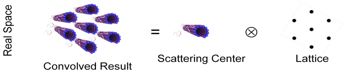
Figure 2.5| A system of scattering centers in a lattice can be mathematically described as the convolution ( \otimes ) of the scattering center with the lattice.
