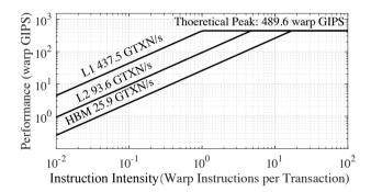
FIGURE 1 Instruction Roofline Model for the GV100. 1 GTXN/s is 10<sup>9</sup> transactions per second.
