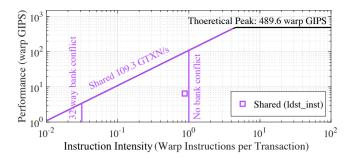
**FIGURE 4** Shared memory walls on the Instruction Roofline plot on GV100. A generic kernel has been plotted on the Roofline for pedagogical purposes. The position of the open dot visualizes the number and impact of bank conflicts.
