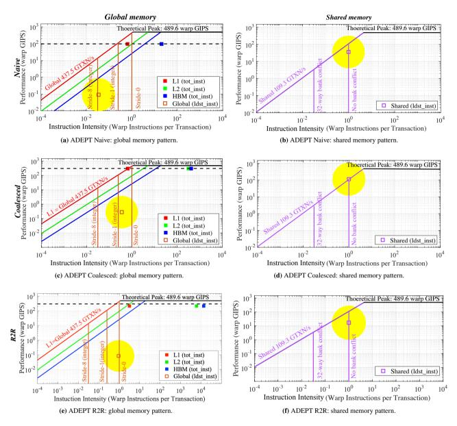
**FIGURE 8** Instruction Roofline on GV100 for the two implementations in ADEPT with visualized global memory pattern. The solid dots are the total number of instructions (tot\_inst) executed by non-predicated threads. The open dots refer to the memory access patterns.
