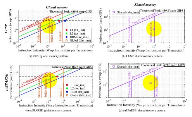
**FIGURE 10** Instruction Roofline on GV100 for the SpMV. The solid dots are the total number of instructions (tot\_inst) executed by non-predicated threads. The open dots refer to the memory access patterns.
