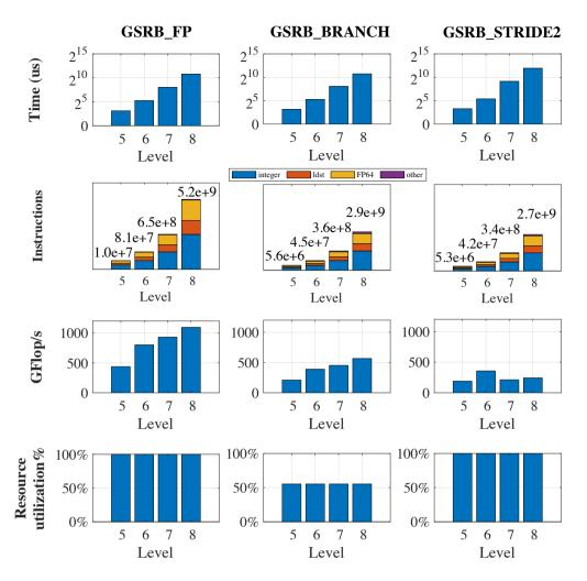
**FIGURE 6** Performance insights breakdown on GV100 for the three different implementations of HPGMG as a function of multigrid level (note, level 8 represents the largest arrays). Resource utilization refers to the ratio of thread predication.
