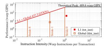
**FIGURE 3** Global memory walls on the Instruction Roofline plot for the GV100. A generic kernel has been plotted on the Roofline for pedagogical purposes. The position of the open dot visualizes the stride of the memory access pattern.
