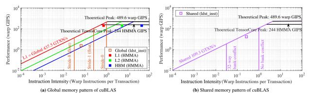
**FIGURE 12** Instruction Roofline on GV100 for the cuBLAS. The solid dots are just HMMA instructions while the open dots are global/share load/store.
