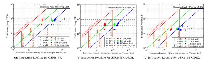
**FIGURE 5** Instruction Rooflines on GV100 for the three implementations of HPGMG's GSRB. Solid dots are the total number of instructions (tot\_inst) executed by non-predicated threads, open dots refer to the global memory access patterns, and dotted lines are warp-level instructions. Note, "level #" refers to the level in the multigrid v-cycle.
