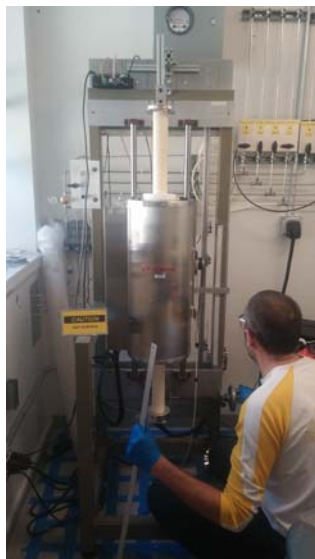
Figure 2.1: A Bridgman furnace I helped to design, in use May 2015
