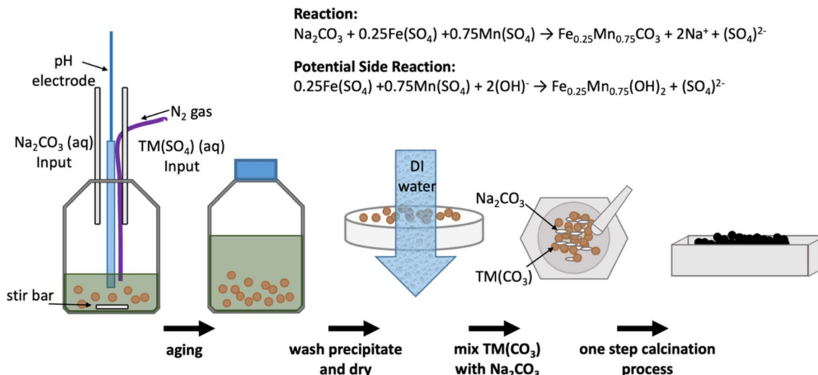
Figure 1. Schematic of the modified co-precipitation synthesis process for meso-structure controlled sodium iron manganese oxide.
