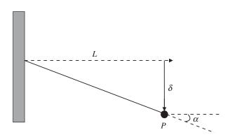
**Figure 3.** A schematic showing the cantilevered beam modelled in this paper. The beam, which consists of the petiole and midrib (together = l), will begin at right angles to the hypothetical trunk, and will deflect downwards ( $\delta$ ) due to the impact of the gecko (*P*). This will result in an angular excursion of the beam ( $\alpha$ ).
