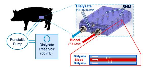
**Figure 6.** SNMHD dialysate recirculation schematic. Dialysate is recirculated from a reservoir and sampled over time. Solute exchange occurs through the SNM interface between the blood and dialysate chambers. Changes in solute concentration allow measurement of normalized SNMHD clearance.
