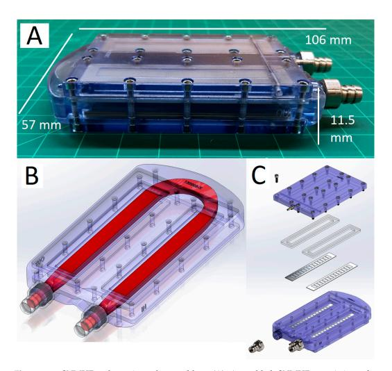
**Figure 5.** SNMHD schematic and assembly. **(A)** Assembled SNMHD consisting of a polycarbonate blood flow housing, SNM, and stainless-steel graft and dialysate connectors (106 mm L  $\times$  57 mm W  $\times$  11.5 mm H). **(B)** CAD image demonstrating blood flow path geometry. **(C)** An exploded view of the SNMHD, showing that the blood path is bordered by parallel SNM and held in place by compressive forces provided by the polycarbonate dialysate manifold and silicone gaskets.
