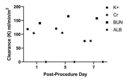
**Figure 4.** SNMHD effectively clears potassium (K+), creatinine (Cr), and urea (BUN) on post-procedure days 1, 5, and 7. No albumin was detected in the dialysate at any of the three timepoints.
